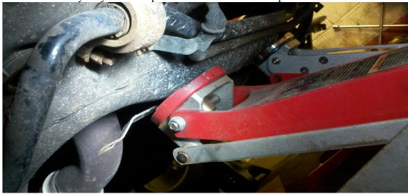
After you have removed both subframe bolts, slowly lower the floor jack so the subframe can drop down. You should now have some room to work as seen in the photo below:
