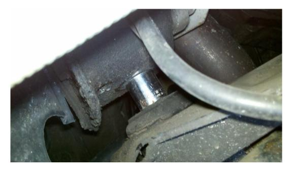
Using the floor jack, jack the subframe up. The socket will pushing the old subframe bushing out as it draws closer and closer until it pops completely out. Clean up any metal shavings you may have and other debris. Make sure all surfaces the bushing will be in contact with are completely clean.
