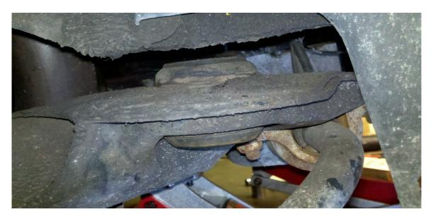
I used a sawzall with a metal cutting blade to make a horizontal cut. Looking at photo #2 above, imagine the blade placed flush against the top of the subframe on the left hand side of the bushing, cutting towards the front of the car (this is the passenger side bushing). With the top of the bushing now cut off, I placed a socket in between the now cut bushing and chassis above it. See the following photo:
